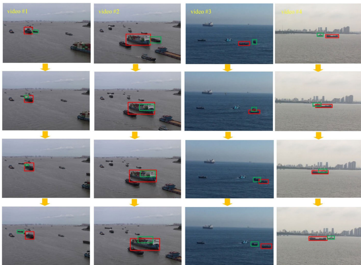
FIGURE 3. Image samples for each collected video clip (green rectangle is the target ship and the red is obstacle).
